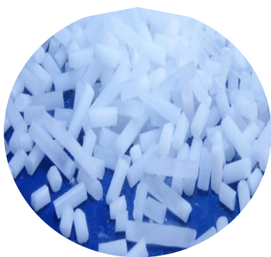
Cleaning with dry grain CO 2 pellets (rice grain 3mm)
