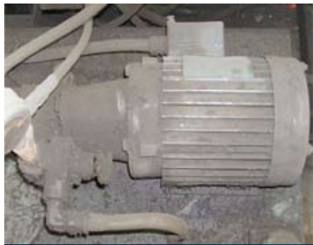
The photos above show the “before” and “after” of a motor cleaned via Precision IceBlast’s IceBlast, a high velocity spray of dry ice.
