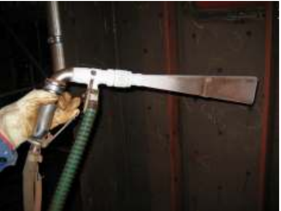
Photo 4 The cleaning nozzle
