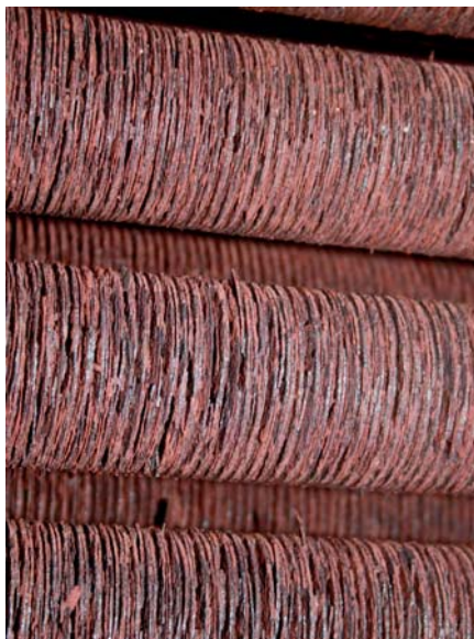
Before and after pictures of the cleaning, using tube spreading process
